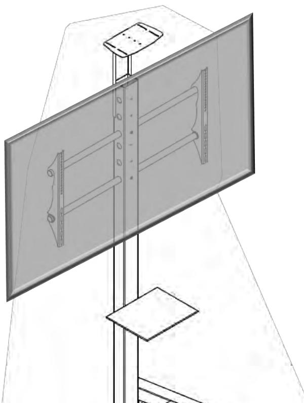
Install the screen on the FIX TROLLEY
