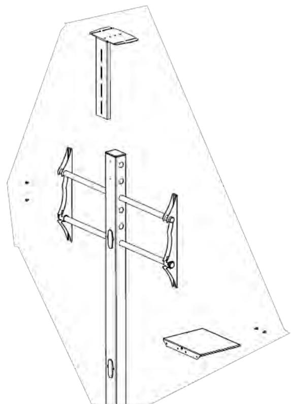
Insert the cables of your monitor inside the tube B through the oval holes and then cover the holes with the cap R
